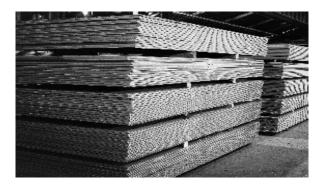
**Hot-rolled plates** are manufactured in a wide range of sizes for applications in several industries varying from construction to pressure vessels and wear-resistant chemistries.
